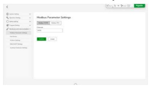
After the connection is established on client side, you can read the Lexium Cobot state and control the Lexium Cobot I/O signal based on the register address and the function code program in the Modbus Address Table, page 227.
