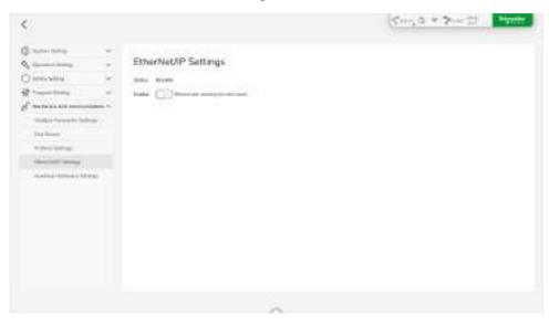
The EtherNet/IP function can be enabled or disabled (default) and can only interact with the external controller for Ethernet/IP communication when enabled. The EtherNet/IP I/O information is displayed in the IO interface.
