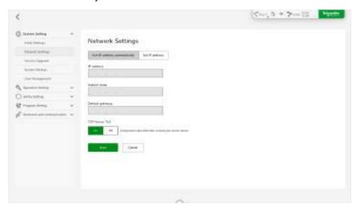
In case the IP address of the Lexium Cobot needs to be set, ensure that the devices communicating with the Lexium Cobot over the network are on the same subnet as the Lexium Cobot.
