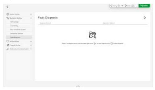
In case of a Lexium Cobot detected error, the Lexium Cobot Controller automatically saves the information in a compressed file named after the system time and displays it in the **Fault Diagnosis** pane.
