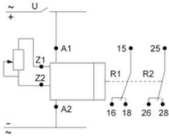
Function K: Delay On De-energization without Auxillary Supply
