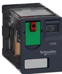
miniature plug in relay, Harmony Electromechanical Relays, 6A, 4CO, without LED, lockable test button, flat (faston type), 120V AC
