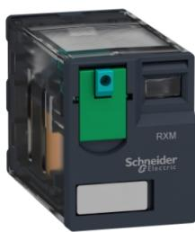
miniature plug in relay, Harmony Electromechanical Relays, 6A, 4CO, without LED, lockable test button, flat (faston type), 110V DC
