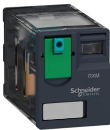
miniature plug in relay, Harmony Electromechanical Relays, 3A, 4CO, without LED, lockable test button, flat (faston type), 24V DC
