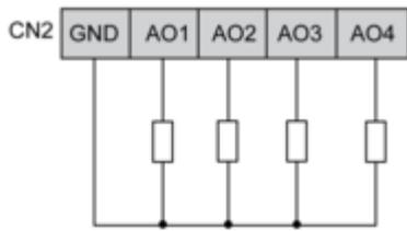
AO3, AO4 can be used also as PWM generator, up to 2kHz.
