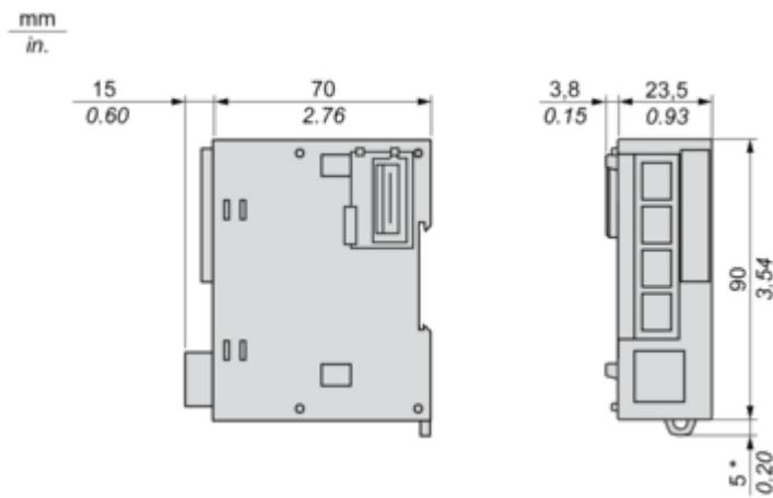
(\*) 8.5 mm/0.33 in when the clamp is pulled out.
