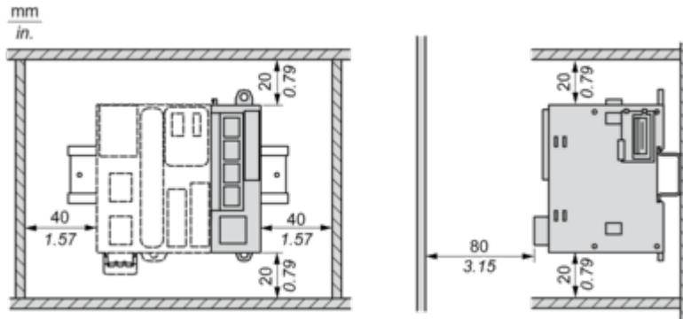
Mounting on a Rail
