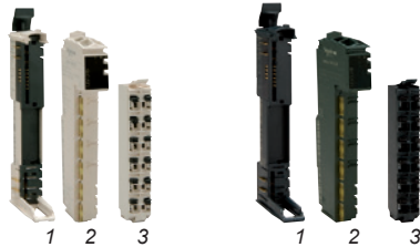
Expansion modules 1 Base 2 Electronic module 3 Terminal block
