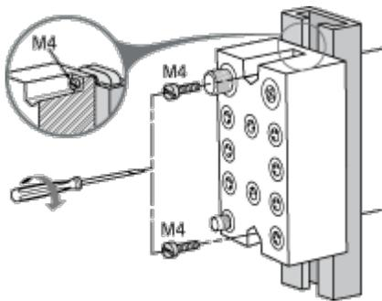
NOTE: Maximum torque to fasten the required M4 screws is 0.6 N.m (5.3 lbf-in).
