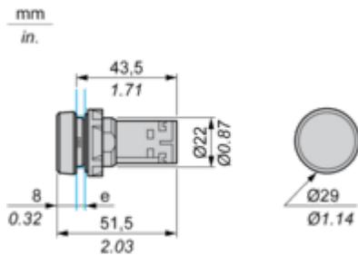
• Support panel thickness: 1 to 6 mm/0.4 to 0.24 in. (metal), 2 to 6 mm/0.8 to 0.24 in. (plastic).
