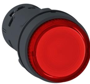
Illuminated push button, Harmony XB7, red projecting, 22mm, integral LED, push and push to release, 1NO, 24V AC
