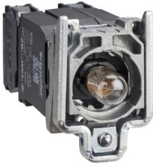
Complete body/contact assembly and light block, Harmony XB4, with body/fixing collar, BA9s incandescent bulb, 220...240V, 1NO + 1NC
