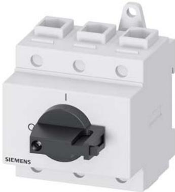
SENTRON, Switch disconnector 3LD, main switch, 3-pole, I<sub>u</sub>: 100 A, Operating power / at AC-23 A at 400 V: 37 kW, installation in distribution boards, knob-operated mechanism, black, handle direct at the switch
