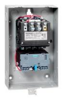
Non-reversing motor starter, Size 1, Three phase full voltage, Solid-state overload relay, OLR amp range 0.75-3.4A, Non-combination type, Enclosure type 1, Indoor general purpose use, Standard width enclosure
