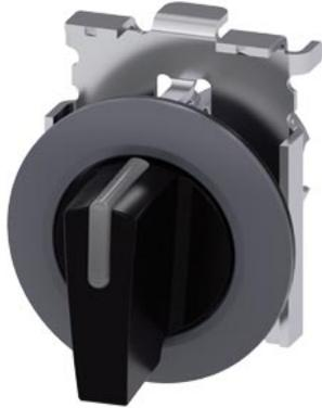
Illuminable selector switch, 30 mm, round, Metal matte, black, Selector switch short, front ring for flush installation, momentary contact type, actuating angle 2x45°, 10:30h/12h/13:30h
