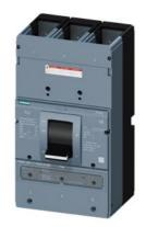
circuit breaker 3VA5 UL frame 1200 breaking capacity class M 35kA @ 480 V 3-pole, line protection TM230, FTAM, In=900A overload protection Ir=900A fixed short circuit protection Ii=5 - 10 x In w/o connection
