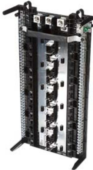
SIEMENS LOW VOLTAGE PL SERIES UNASSEMBLED LOAD CENTER. MAIN LUG INTERIOR WITH 30 1-INCH SPACES ALLOWING MAX 54 CIRCUITS. 3-PHASE 4-WIRE SYSTEM RATED 120/240V OR 120/208V (200A) 100KA INTERRUPT. SPECIAL FEATURES: COPPER BUS, INTERCHANGEABLE MAIN.
