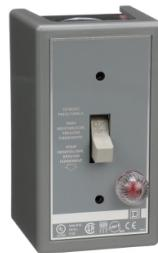
Manual Starter, fractional horsepower, 16A, 1 pole, 1 HP at 277 VAC, toggle operated, green indicator, NEMA 1 enclosure
