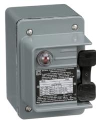
Manual Starter, fractional horsepower, 16A, 1 pole, 1 HP at 277 VAC, red indicator, NEMA 4 enclosure, 1 conduit opening
