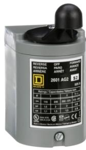
Switch, reversing drum, 2 HP at 230 VAC single phase, 2 HP at 575 VAC polyphase, handle operated, NEMA 1 enclosure
