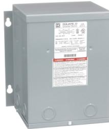
Transformer, dry type, encapsulated, 2kVA, 1 phase, 240x480V primary, 120/240V secondary, 9A, 115C rise [TAA]
