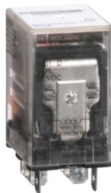
Miniature Relay, Harmony 8501R, DPDT, 8 blades, coil, green, LED, 15A resistive at 120V AC, 1HP at 277V AC, 24V DC, 2NO + 2NC
