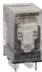
Plug in relay, Type R, miniature, 1 HP at 277 VAC, 15A resistive at 120 VAC, 8 blade, DPDT, 2 NO, 2 NC, 24 VDC coil
