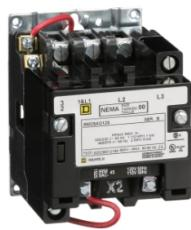
NEMA Contactor, Type S, nonreversing, Size 00, 9A, 3HP at 575VAC, 3 phase, up to 100kA, 3 pole, 120VAC coil, open [TAA]
