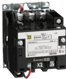
NEMA Contactor, Type S, nonreversing, Size 0, 18A, 2HP at 230VAC, 1 phase, up to 100kA, 2 pole, 120VAC coil, open [TAA]
