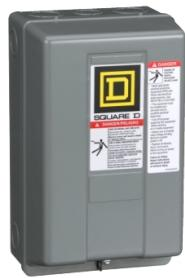
NEMA Contactor, Type S, nonreversing, Size 1, 27A, 10HP at 575VAC, 3 phase, up to 100kA, 3 pole, 120VAC coil, NEMA 1 [TAA]
