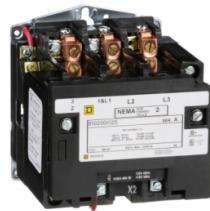
NEMA Contactor, Type S, nonreversing, Size 2, 45A, 25HP at 575VAC, 3 phase, up to 100kA, 3 pole, 208VAC coil, open [TAA]
