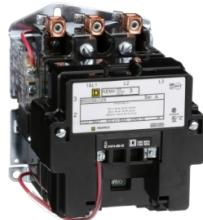
NEMA Contactor, Type S, nonreversing, Size 3, 90A, 50 HP at 575 VAC, 3 phase, up to 100 kA, 3 pole, 120 VAC coil, open [TAA]
