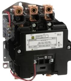
NEMA Contactor, Type S, nonreversing, Size 4, 135A, 100 HP at 575 VAC, 3 phase, up to 100 kA, 3 pole, 120 VAC coil, open [TAA]
