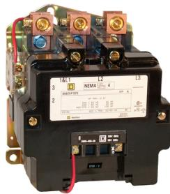
**NEMA Contactor, Type S, nonreversing, Size 4, 135A, 100HP at 575VAC, 3 phase, up to 100kA, 3 pole, 480VAC coil, open [TAA]**
