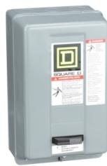
NEMA motor starter, Type S, nonreversing, Size 00, 9A, 2HP at 460VAC, 5kA SCCR, 3 phase, 3 pole, melting alloy, 120VAC coil, NEMA 1 [TAA]
