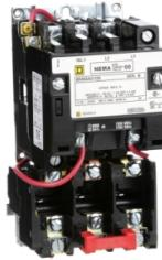
NEMA motor starter, Type S, nonreversing, Size 00, 9A, 2HP at 460VAC, 5kA SCCR, 3 phase, 3 pole, melting alloy, 120VAC coil, open [TAA]
