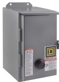
NEMA Motor Starter, Type S, nonreversing, Size 0, 18A, 5 HP at 460 VAC, 5 kA SCCR, 3 phase, 3 pole, melting alloy, 120 VAC coil, NEMA 12 [TAA]
