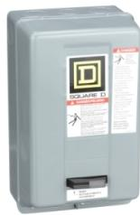
NEMA motor starter, Type S, nonreversing, Size 0, 18A, 5HP at 460VAC, up to 100kA SCCR, 3 phase, 3 pole, Motor Logic, 120VAC coil, NEMA 1 [TAA]
