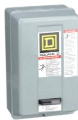
NEMA motor starter, Type S, nonreversing, Size 0, 18A, 5HP at 460VAC, 5kA SCCR, 3 phase, 3 pole, melting alloy, 120VAC coil, NEMA 1 [TAA]
