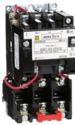
NEMA Motor Starter, Type S, nonreversing, Size 0, 18A, 5 HP at 460 VAC, 5 kA SCCR, 3 phase, 3 pole, melting alloy, 24 VAC coil, open [TAA]
