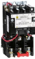
NEMA motor starter, Type S, nonreversing, Size 0, 18A, 5HP at 460VAC, 5kA SCCR, 3 phase, 3 pole, melting alloy, 120VAC coil, open [TAA]
