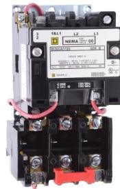
NEMA motor starter, Type S, nonreversing, Size 0, 18A, 5HP at 460VAC, 5kA SCCR, 3 phase, 3 pole, melting alloy, 240VAC coil, open [TAA]
