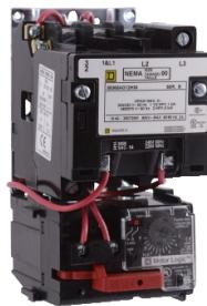
NEMA Motor Starter, Type S, nonreversing, Size 0, 18A, 5 HP at 460 VAC, up to 100 kA SCCR, 3 phase, 3 pole, Motor Logic, 240 VAC coil, open [TAA]
