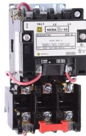
NEMA motor starter, Type S, nonreversing, Size 0, 18A, 5HP at 460VAC, 5kA SCCR, 3 phase, 3 pole, melting alloy, 480VAC coil, open [TAA]
