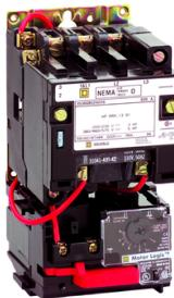
NEMA Motor Starter, Type S, nonreversing, Size 0, 18A, 5 HP at 460 VAC, up to 100 kA SCCR, 3 phase, 3 pole, Motor Logic, 208 VAC coil, open [TAA]
