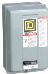
NEMA Motor Starter, Type S, nonreversing, Size 1, 27A, 10 HP at 460 VAC, 5 kA SCCR, 3 phase, 3 pole, melting alloy, 24 VAC coil, NEMA 1 [TAA]
