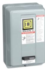
NEMA motor starter, Type S, nonreversing, Size 1, 27A, 10HP at 460VAC, 5kA SCCR, 3 phase, 3 pole, melting alloy, 240VAC coil, NEMA 1 [TAA]
