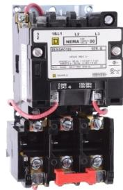
NEMA motor starter, Type S, nonreversing, Size 1, 27A, 10HP at 460VAC, 5kA SCCR, 3 phase, 3 pole, melting alloy, 480VAC coil, open [TAA]
