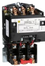
NEMA motor starter, Type S, nonreversing, Size 2, 45A, 25HP at 460VAC, 5kA SCCR, 3 phase, 3 pole, melting alloy, 120VAC coil, open [TAA]
