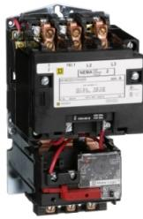
NEMA motor starter, Type S, nonreversing, Size 2, 45A, 25HP at 460VAC, up to 100kA SCCR, 3 phase, 3 pole, Motor Logic, 480VAC coil, open [TAA]
