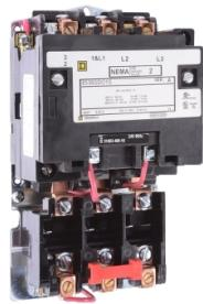
NEMA Motor Starter, Type S, nonreversing, Size 2, 45A, 25 HP at 460 VAC, 5 kA SCCR, 3 phase, 3 pole, melting alloy, 208 VAC coil, open [TAA]
