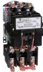
NEMA motor starter, Type S, nonreversing, Size 3, 90A, 50HP at 460VAC, 5kA SCCR, 3 phase, 3 pole, melting alloy, 480VAC coil, open [TAA]
