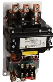
NEMA motor starter, Type S, nonreversing, Size 5, 270A, 200HP at 460VAC, 10kA SCCR, 3 phase, 3 pole, melting alloy, 120VAC coil, open [TAA]
