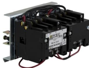
NEMA Contactor, Type S, reversing, horizontal, Size 0, 18A, 5HP at 575VAC, 3 phase, up to 100kA, 3 pole, 120VAC coil, open style [TAA]
